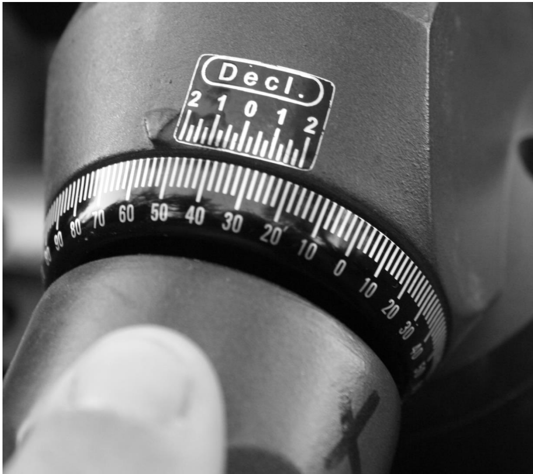
Figure 14: Meade LXD55 DEC Setting Circle a Little Over 2 Inches in Diameter
