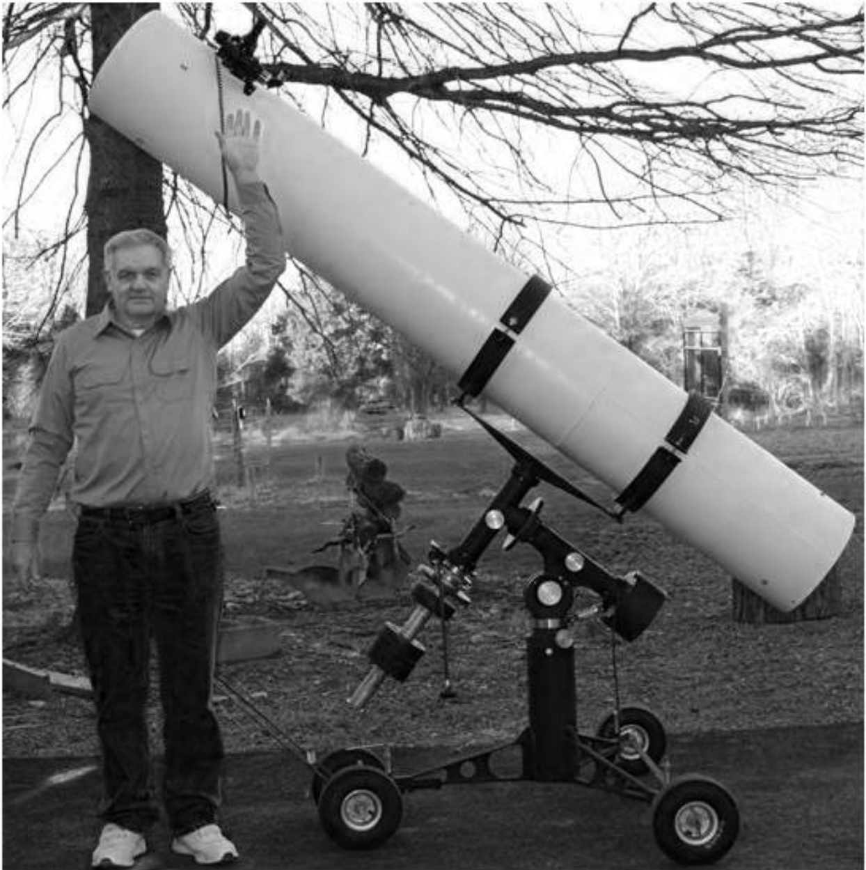
Figure 10: My 12 ½ inch, f/8, Newtonian, on a Starliner Equatorial Mount with 2 Inch Shafts (Tube is 9 ft. in Length, 15 in. OD, OTA Weight 57 lbs.)
