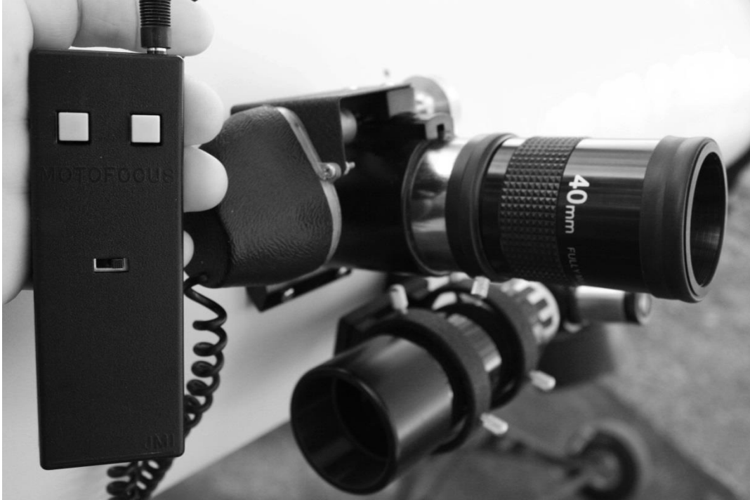
Figure 12: Electronic Focusing Controller and Drive Unit on my 12 ½ inch, f/8, Newtonian, with a 2 Inch OD, 40 mm fl Eyepiece in the Focuser and a 50 mm Finder Scope nearby
