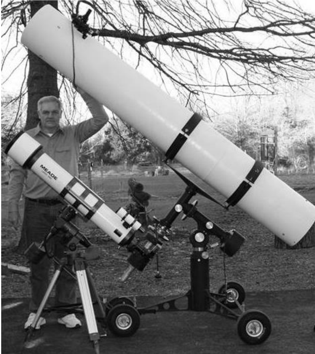
Figure 13: Meade LX200 Mount with 6-inch Refractor Compared to my 12 ½ inch, f/8, Newtonian, on my Starliner Equatorial
